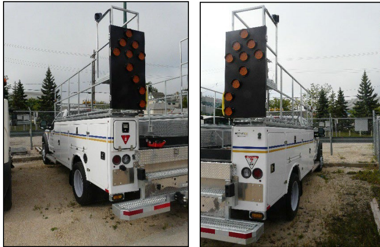
Arrow board incorporated mounting on frame of catwalk
